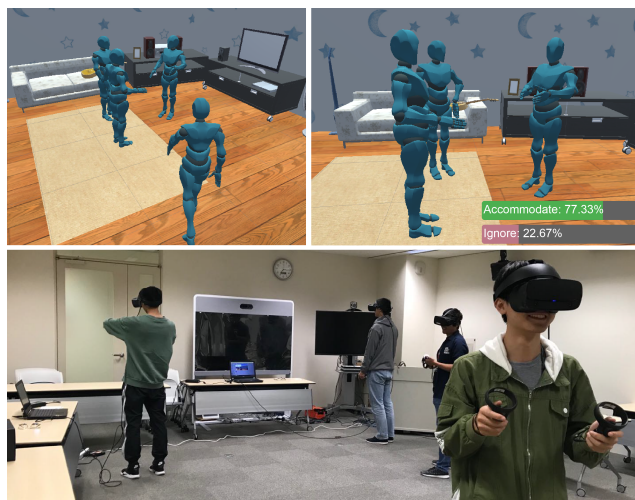
Figure 7: The virtual reality use case. The perspective view of the multi-agent interaction scenario, where a newcomer approaches to join a conversational group (top-left). The first-person view of the newcomer with the normalized probability of group behaviors represented by color bars (top-right). Each participant controls one virtual character with one VR device (bottom).
