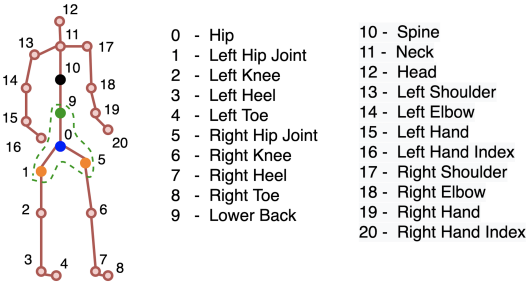
Fig. 3: The spatial graph of a skeleton used in this work. Each graph node corresponds to the marker on the right [42]. The edges between nodes are defined based on natural joints relationships.
